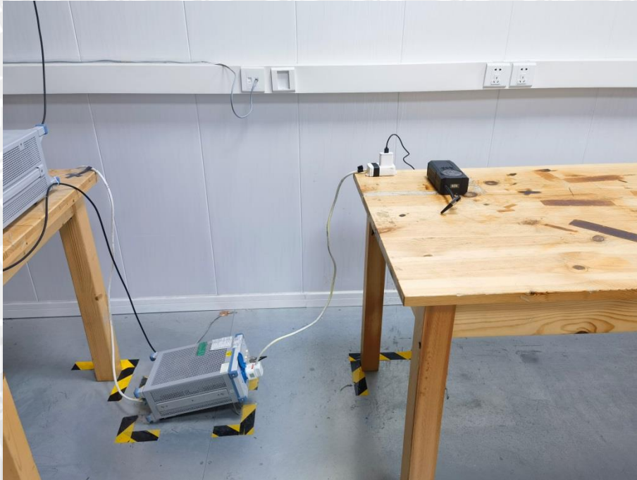
Photograph 1: Set-up for Disturbance Voltage
