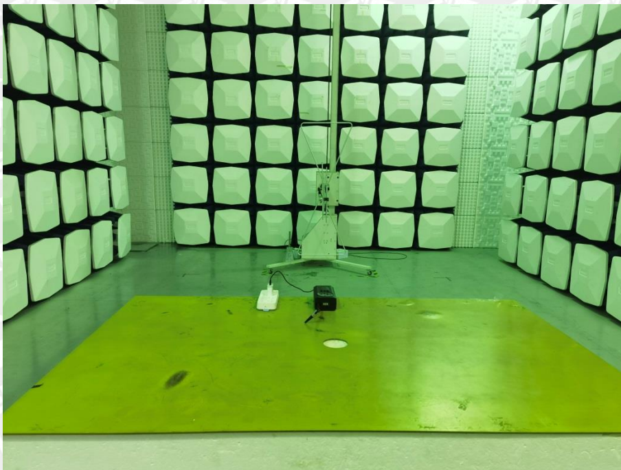
Photograph 2: Set-up for Radiated Emission
