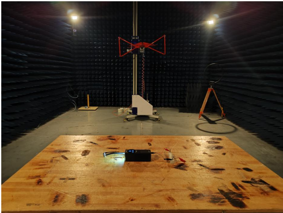
Radiated Test Setup Photograph
