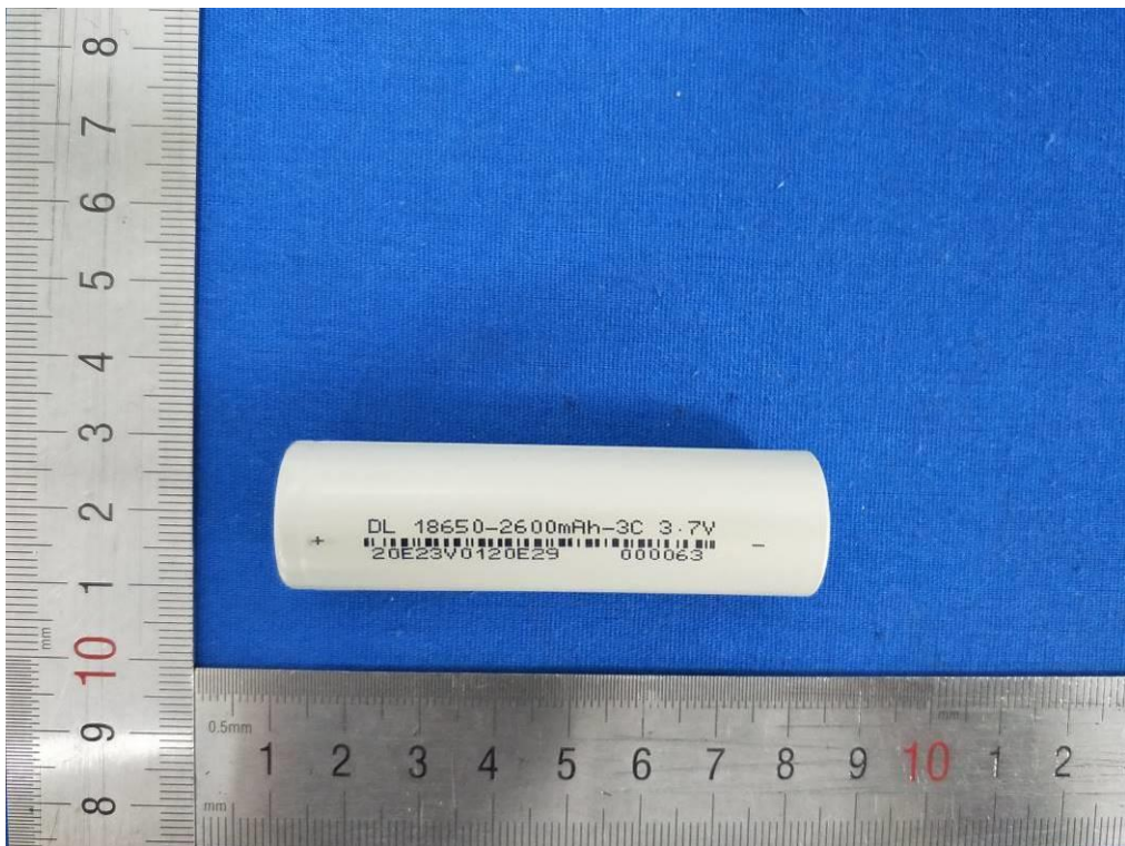
Figure 6 Terminal view of cell (DL 18650-2600mAh-3C)
